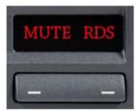
To mute the volume press the left key when this is in the display. To turn off the mute press the left key again.
